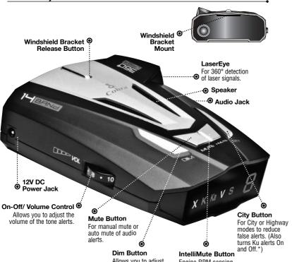
Allows you to adjust the UltraBright Data Display brightness for easy reading. (Also turns VG-2 and Spectre I & IV+ alerts On and Off.\*)
