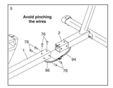
Locate the wire tie in the top of the Upright (2) and pull the Upper Wire (94) out of the Upright. Then, untie and discard the wire tie.
