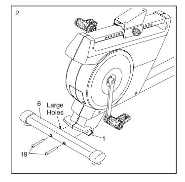
3. Orient the Upright (2) and the Front Stabilizer (5) so that the large holes are facing the Upright.
