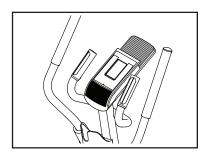
To insert a tablet or smart phone into the tablet holder, set the bottom edge of the tablet or smart phone in the tray. **Make sure that the tablet or smart phone is firmly secured in the tablet holder.** Reverse these actions to remove the tablet or smart phone from the tablet holder.
