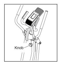
Then, lift a pedal, fold the brace upward, and pivot the pedal downward to the low position. **Repeat this** action for the other pedal.
