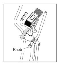
Next, lift a pedal, unfold the brace, and insert the end of the brace into the pedal arm. **Make sure that the brace is securely inserted into the pedal arm. Repeat this action for the other pedal.**
