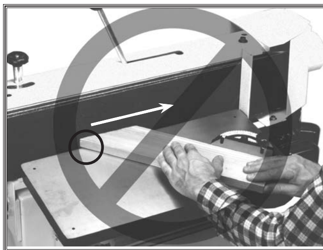
Figure 48. DO NOT sand wood with sharp corners at the leading-edge of the sanding operation. The belt can grab and throw the wood.
