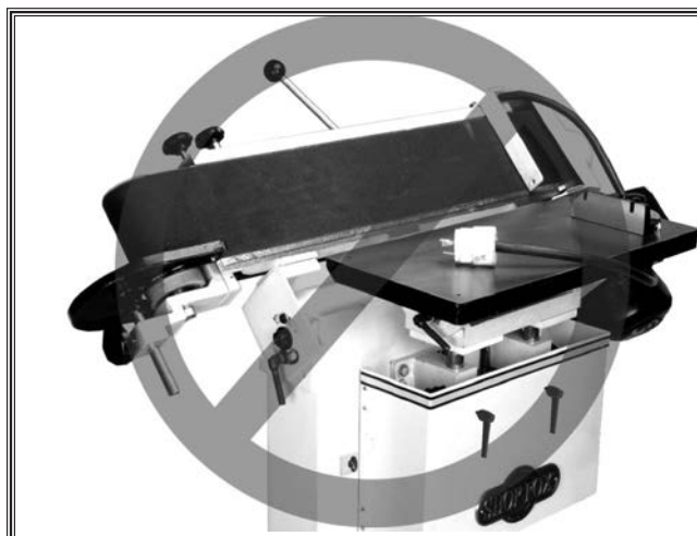
Figure 45. Incorrect platen tilted position.
