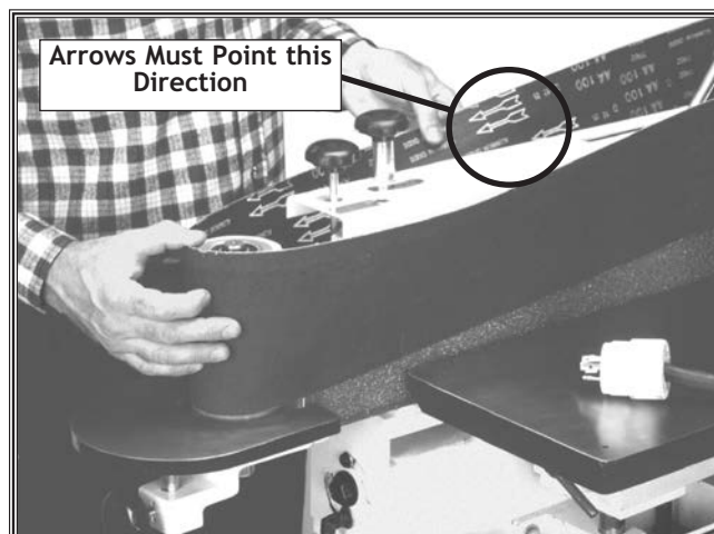
Figure 22. Sanding belt directional installation.
