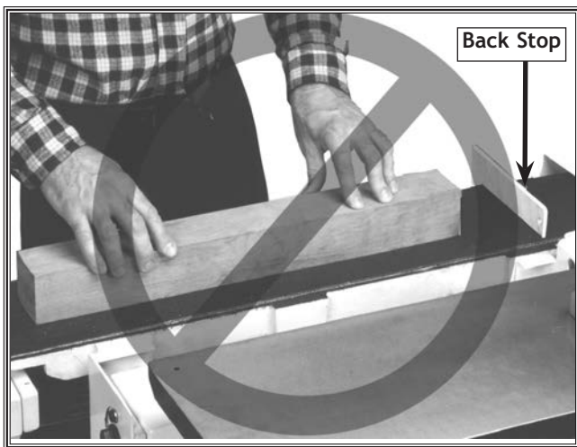
Figure 51. Incorrect face sanding away from back stop.
