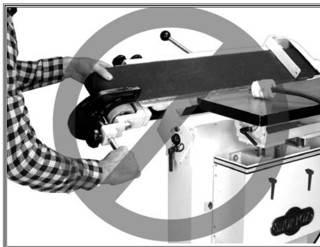
Figure 43. Incorrectly holding and tilting the platen.
