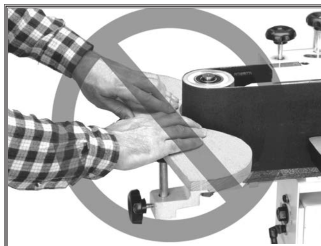
Figure 54. DO NOT sand wood with your fingers close to the idler roller and belt.
